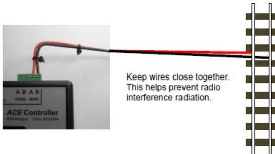
*(The exact method of connecting the wires to the track section, or your layout, will vary in accordance with your setup and preferences. However, we recommend that all wiring to track rails is soldered for reliability.)*
