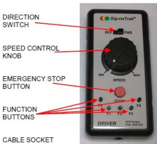
The *DRIVER* handset (part no: BHS1204) provides a low-cost means of adding up to four additional operators and/or giving a more traditional “knob and switches” method of control. A *DRIVER* can be plugged into any of the A, B, C or D sockets on the rear panel of the *ACE*, using the supplied cable.
