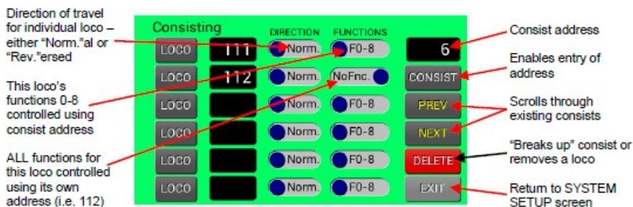
In the above case, an example consist has been previously set up (from this screen). A newly-supplied ACE will display all loco and consist number boxes blank.
