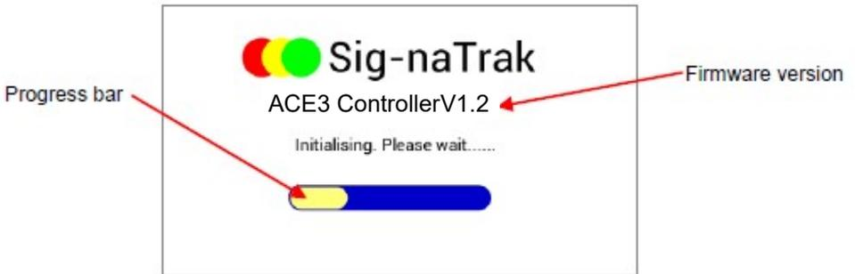
The *ACE* will perform various internal tasks, turn on the *MAIN TRACK* power and then display then *PANEL DRIVE* screen:-
